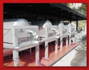
Pressing lines with continuous press system and remote control intergation
