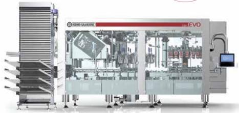
Feeding, dispensing and application of tin and polylaminate capsules (spinning heads) and PVC/PET ones (thermo-shrinking heads).
