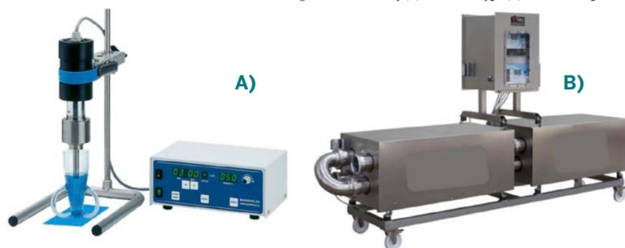
Figure 1. Laboratory (A) and Prototype (B) ultrasound plant
