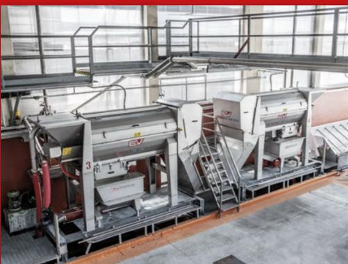
Destemming and crushing lines for both manual or mechanical harvest
