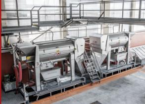
Destemming and crushing lines for both manual or mechanical harvest
